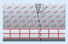
8 | If the sheet width of Exolon® multi UV sheets has to be reduced, please cut as close as possible to the next web to ensure the best clamping action of the glazing bar.
