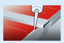
**14** | Seal the upper sealing strip of the end-closure section with silicone rubber that is compatible with Exolon® and smoothen it out so that no water can enter
