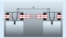
**4** | The clear width or sheet width (B) of Exolon® multi UV sheets is calculated from the rafter spacing, the dimensions of the chosen glazing bars and the required allowance for expansion (3 mm/m for polycarbonate).
