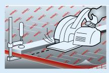
**6** | Marking should be done with a soft crayon on the masking film, which should be left on the sheet during machining and until the sheet has been installed. For cutting, use conventional circular saws with unset, multi-tooth carbide-tipped blades. Always work with a stop.
