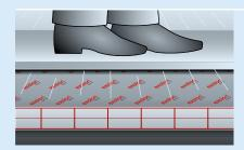
11 | Place the Exolon® multi UV sheets on the purlins. It is important to place the side with UV protection facing outwards or upwards. This side is marked on the masking film and stamped along the sheet edge. Avoid walking on the sheets. If necessary, place a thick plank across the sheet.
