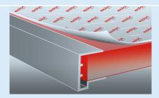
10 | When sealing sheet ends there is a simple, but very important, rule to follow which keeps condensation to a minimum: seal as tightly as possible at the top (e.g. seal edges with aluminium tape and if necessary affix an aluminium-end profile, possibly with seal), and as tight as necessary at the
