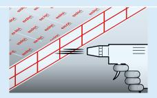
**7** | Swarf that has entered the sheet chambers can be blown out with compressed air or removed using a vacuum cleaner.
