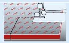
**9** | Corner cutouts are often required (e.g. for pipes, ventilation etc.). Use a jig saw without pendulum action. Drilling can be performed with twist drills (point angle  $\phi$  110°-130°), conical or step drills.
