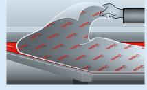
**13** | Finally, remove the masking film from the Exolon® multi UV sheets. It should not be exposed to weathering for more than 24 hours.
