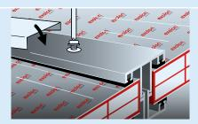
**12** | Peel back the masking film and fasten the upper sections of the glazing bars using the recommended screws with washers. Depending on the glazing system, a cover section is then clipped on.
