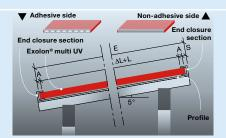
**5** | The correct order length (L) of Exolon® multi UV sheets can be simply and safely determined, bearing in mind the following:
