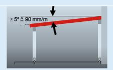
**2** | We recommend a roof pitch of at least  $5^{\circ}$  ( $\triangleq 90 \text{ mm/m}$ ) to allow rainwater to flow off better. This has the benefits of maintaining seal integrity and the sheets are naturally cleaned by the rain.
